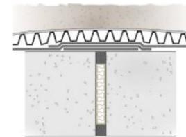
When sealing joints in water tank roofs it is not always practical to install a centrally placed waterstop. An externally placed bandage strip such as Fosroc Expoband H45 is ideal for this application. **Hydrocell XL** joint filler board and **Nitoseal MS600** joint sealants complete the system.
