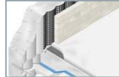
For BS8102:2009 Type C internal drained cavity waterproofing, the structural concrete is designed to minimise water penetration and a suitable HDPE studded drainage membrane is installed to collect groundwater seepage. The groundwater is then directed to suitable discharge points. **Proofex Cavitydrain 80** and **200** drainage membranes can provide up to 10L/s/m water flow capacity.
